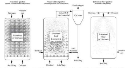
Figure 2: DIFFERENT TYPE OF THERMAL GASIFICATION TECHNOLOGY
